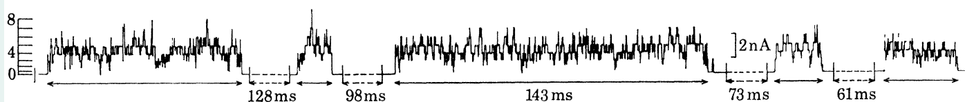
FIGURE 3. Current fluctuations for the membranes of figure 1 in KCl ( 2 \text{ mol dm}^{-3} ) with alamethicin (nominally 10^{-7} \text{ mol dm}^{-3} ) on the negative side. The applied potential was -220 \text{ mV} .
